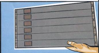
Take 1 Eziblank (R) panel and select the number of rows required. Grasp the underside of the panel at the row division required.
