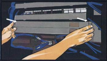
Bend the panel in the opposite direction until it has cleanly snapped off.
