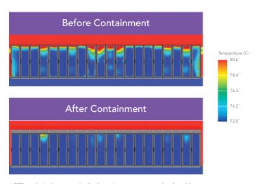
CFD analysis shows evenly distributed temperatures and reduced hot spots after the installation of Rack Top Angle Baffles in the cold aisle.
